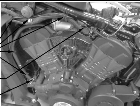
FIGURE 6 (INJECTOR & FRONT O 2 HARNESS ROUTING LOCATIONS)
