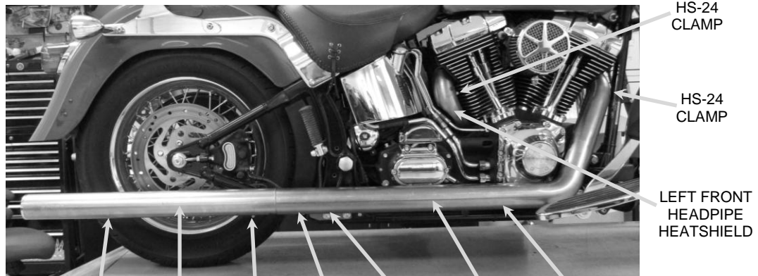
NOTE: Arrows point to the position of the hex head of the clamps. HS-28 CLAMP RIGHT MUFFLER HEATSHIELD HS-28 CLAMP 27-61MSC CLAMP HS-24 CLAMP RIGHT FRONT HEADPIPE HEATSHIELD HS-24 CLAMP
